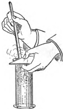
Fig. 15.—Testing oxygen with burning splinter.
